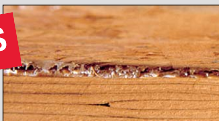
Standard Water or Solvent Based Subfloor and Construction Adhesives – Rigid with Poor Structural Stability
